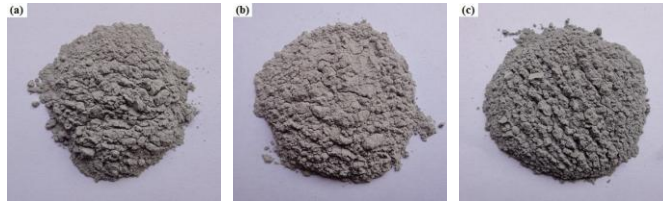
Figure 2. The cement clinker of calcium aluminosilicate slag obtained by crushing and screening.
