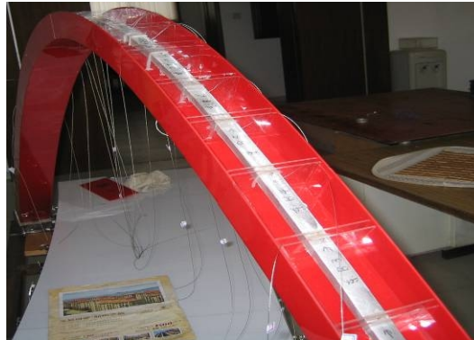
Figure 2 Arch rib core beam and coat
