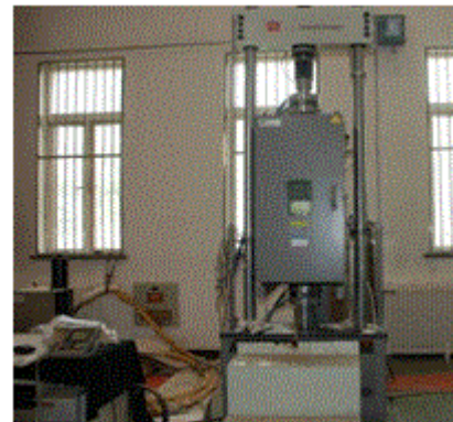
Fig.6 high and low temperature environmental chamber of MTS810
