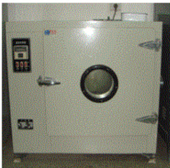
Fig.3 Xenon lamp aging chamber of SN-900
