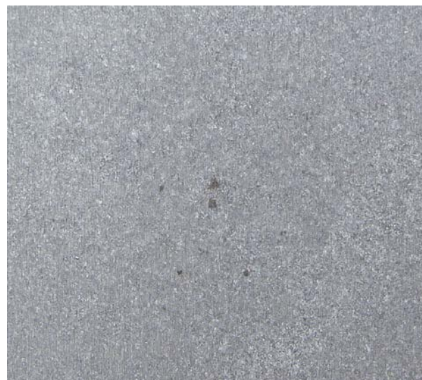
Fig. 1. Macrostructure of steel billet
