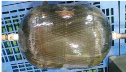
Fig. 1 Picture of the 56 L cryogenic COPV
