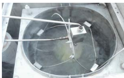
Fig. 16 Test apparatus of pressure- circulation experiment under the temperature of liquid nitrogen
