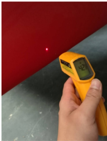
(a) Temperature measuring probe
