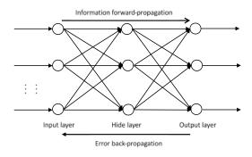
Fig. 1. Three-layer BP network model
