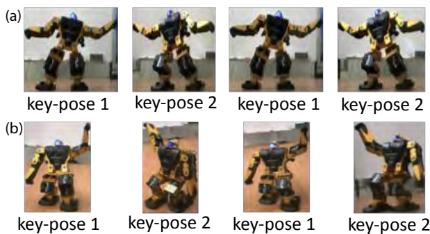
Figure 5: Key-poses of the two dance movements used in the quantitative and qualitative evaluations of the system: (a) mov1 ; (b) mov2 .
