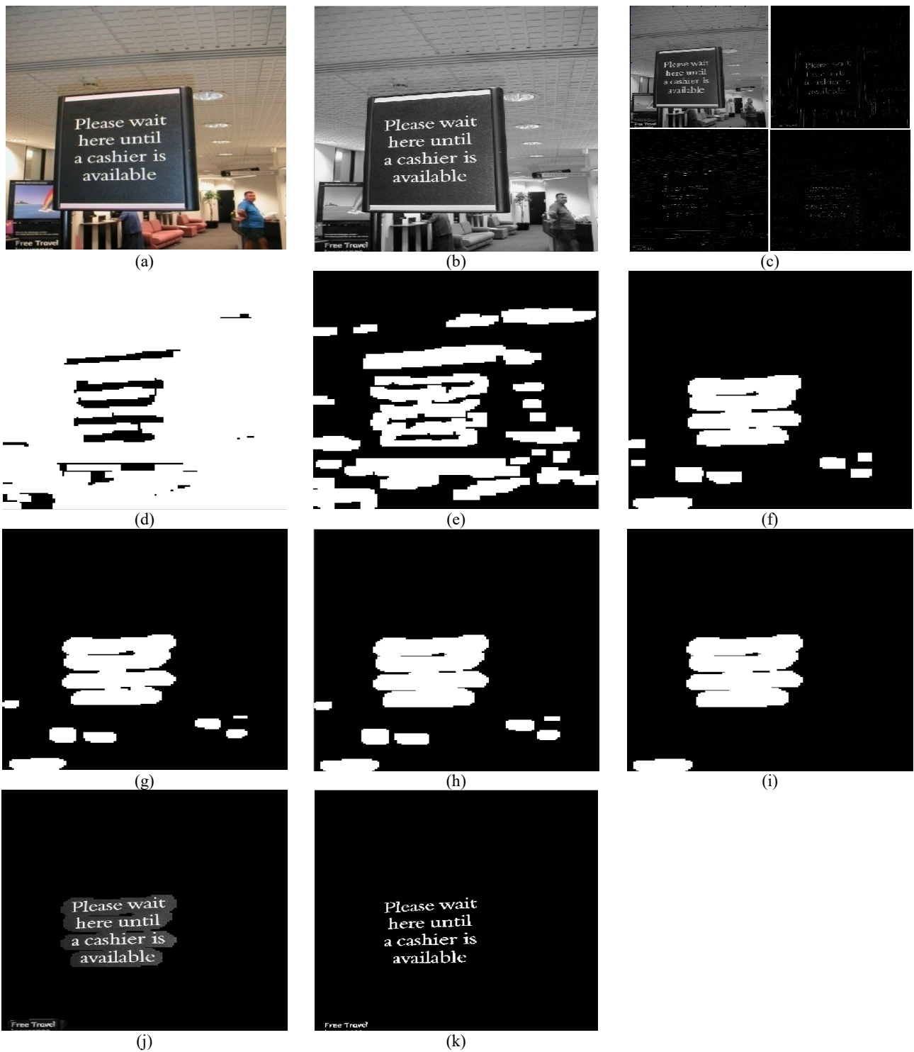
Fig. 5: Steps involved in text extraction for complex background image: (a) input color image; (b) pre-processing; (c) 2D DWT; (d) simple background cluster; (e) complex background cluster; (f) text cluster; (g) masked image; (h) morphological dilation operation; (i) removal of non-text regions (area-based filtering); (j) extracted text; (k) refining of text region
