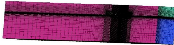
Fig. 3. General view of the volume mesh of the computational domain
