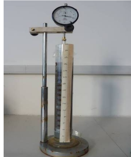
Fig. 4 Water Retention Behavior Fig. 5 Self-made Dilatation Rate Measuring Device
