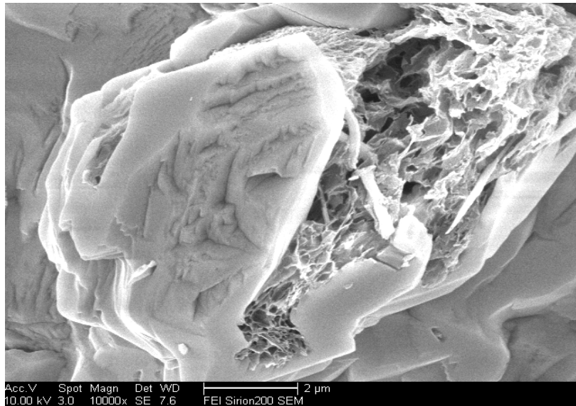
Fig. 1 Poly-Phase Cellular Structure of hardenite of High Water Retention and Dilatation Material Dilatation Mechanism
