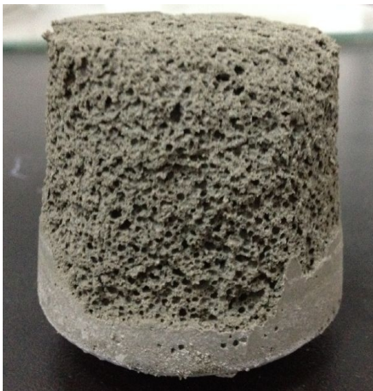
Fig. 2 is what the dilatation of the backfill was like when foam agent are 0.8% of cementing material
