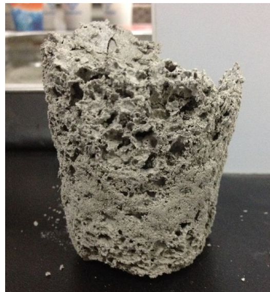
Fig. 3 is what the dilatation of the backfill was like when foam agent are 1.7 % of cementing material
