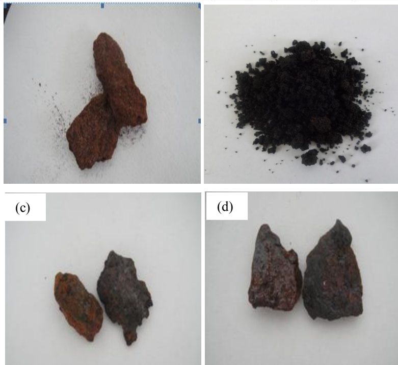
Fig.2 Scale morphology of typical oil wells (a) C33-28 well (b) C80-19 well (c) C19-213well (d) C31-136 well
