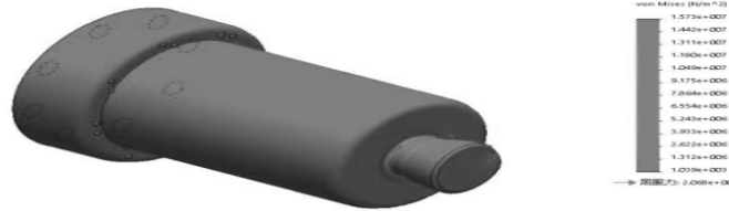
Fig.6 stress distribution pattern of driving force transmission mechanism
