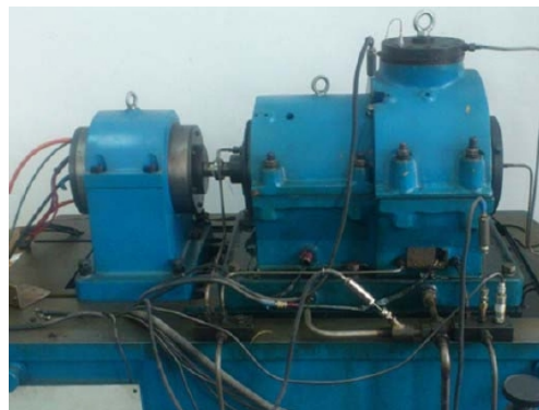
Fig.6 Cage dynamic performance test rig for aero-bearing
