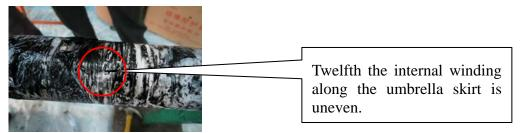
The disintegration of layers of dig inspection found sixth small holes along the wall bushing, Ninth edge from the outside to the inside of the three layer capacitive discharge, sixth, ninth and twelfth along the 90 degree angle from the outside to the inside of the two layer capacitive discharge. (as shown below)
