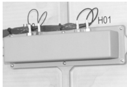
Fig. 8 Shielding Structure with Feed-through Capacitor
