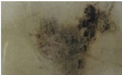
Fig. 5 discharge trace of inner insulation paperboard
