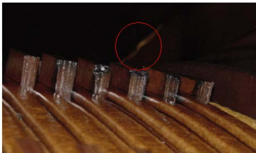
Fig. 3 discharge position of coil gasket
