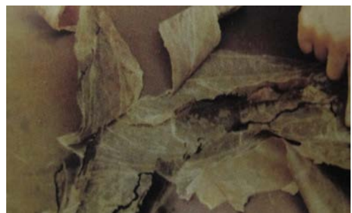
Fig. 6 large area dendritic discharge
