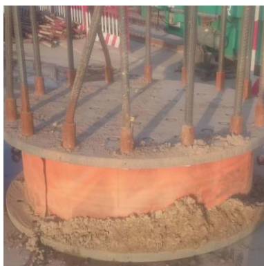
Fig. 7. Storage location and other issues lead to the corrosion of the bearing
