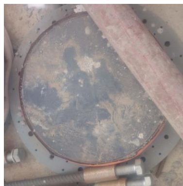
Fig. 8. PTFE is contaminated
