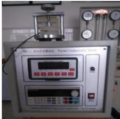
Fig.3 DRE-III multifunction rapid thermal conductivity tester
