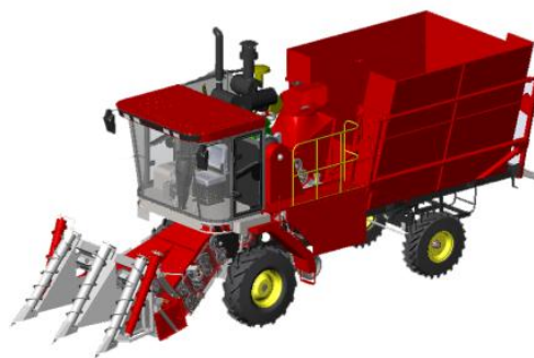
Figure 1. The double-rows sugarcane harvester
