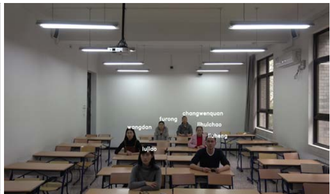
Figure 2 Result of face detection by Faster R-CNN. Figure 3 Face identification result of SeetaFace.
