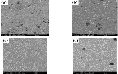
Fig. 4 Microstructure of TiC-TiB<sub>2</sub> ceramics with different Ni mass fraction FESEM (a)5% (b) 10% (c)15% (d) 20%
