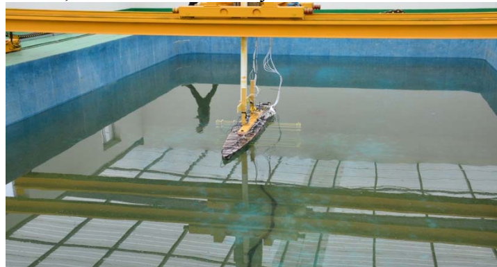
Fig. 6 Scaled ship model and underwater measuring device
