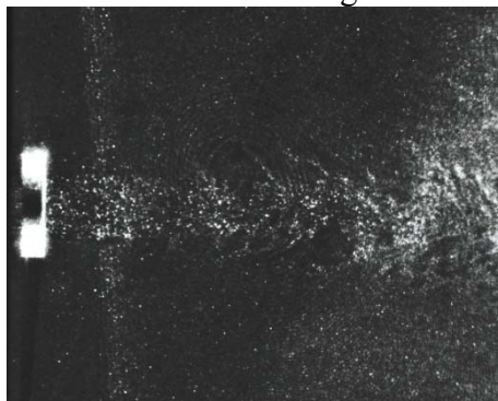
Fig.5 Scattering Image of Particles from Free-jet Experiment
