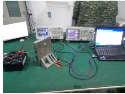
Fig. 2 Channel gain magnitude measurement Experimental setup
