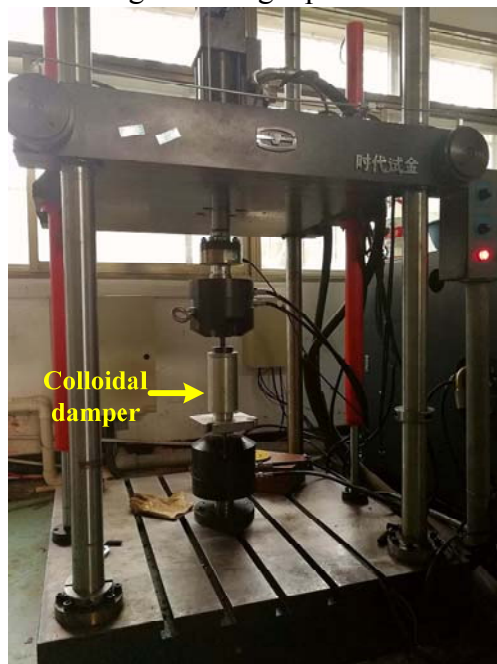
Fig.6 Colloidal damper and test rig
