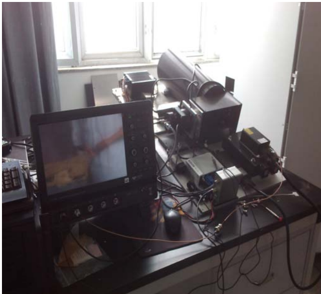
Fig. 1. Multi-wavelength polarization lidar system and debugging in the lab.
