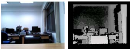
FIGURE II. THE RGB IMAGE AND DEPTH IMAGE OF ASTRA3D SENSOR
