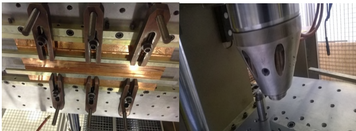
Fig. 1 The experimental setup showing the clamping fixture and the backing plate system and pinless tool used for the experiments.
