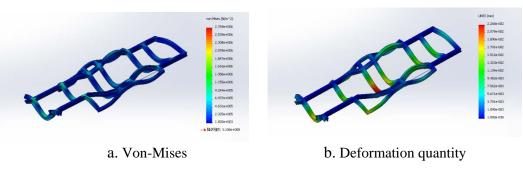
Figure 4 The calculation results of Aluminum base frame
