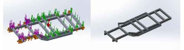
Figure 1 Boundary condition of Base frame model Figure 2 Mesh of Base frame model
