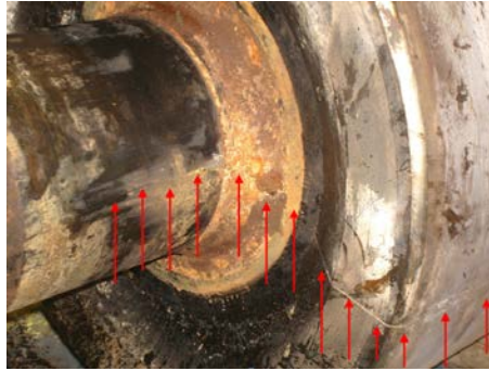
Fig.3. Crack in fitting zone / bearing mounting area
