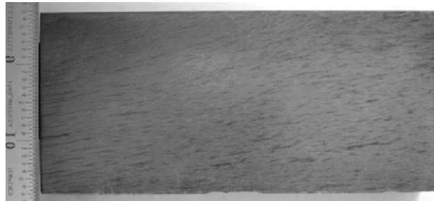
Fig.11. Shaft neck longitudinal macro corrosion test specimen
