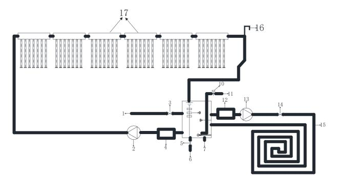
Figure 1. Structure drawing of photo-thermal water-cycling system
