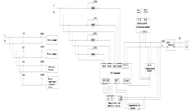
Figure 2. Electric drawing of the control system
