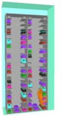
Fig. 6a Transient profile of fire flow at 171 s
