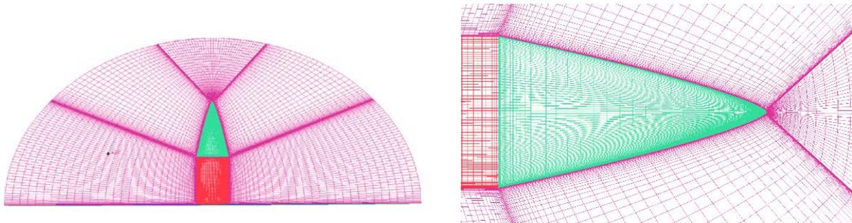
Figure 2 Structural mesh of outflow field
