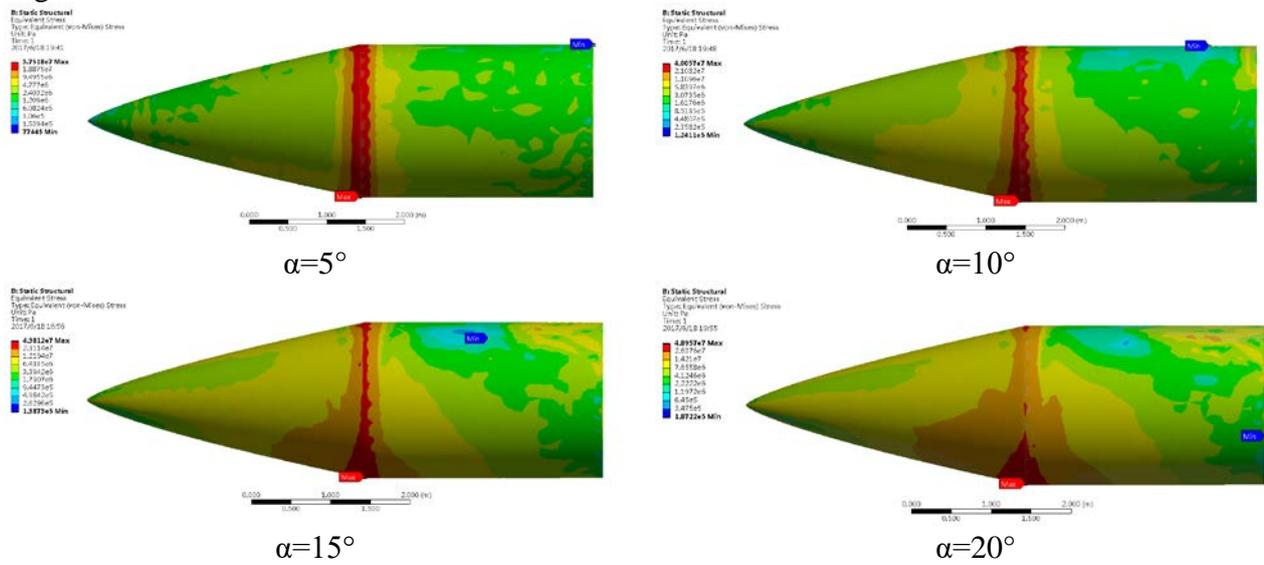
Figure 7 Stress distribution under different attack angles
