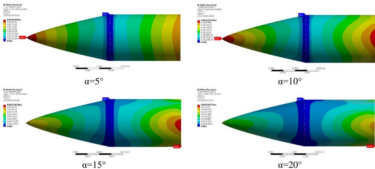
Figure 8 Deformation distribution under different attack angles
