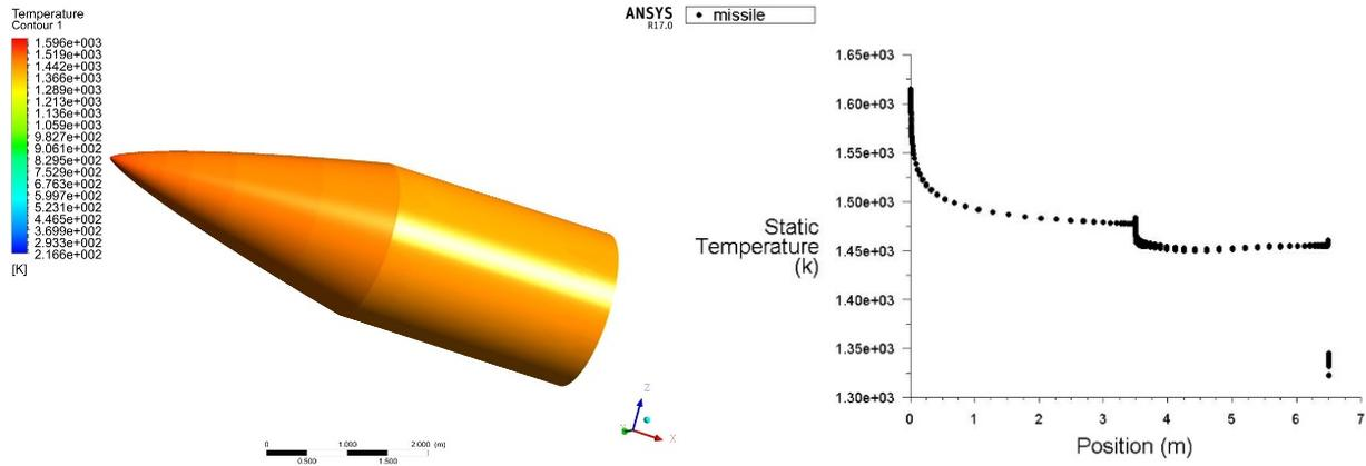
Figure 5 The distribution of flow field temperature
