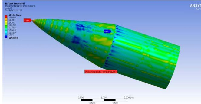
Figure 6 Temperature field of quartz ceramic radome
