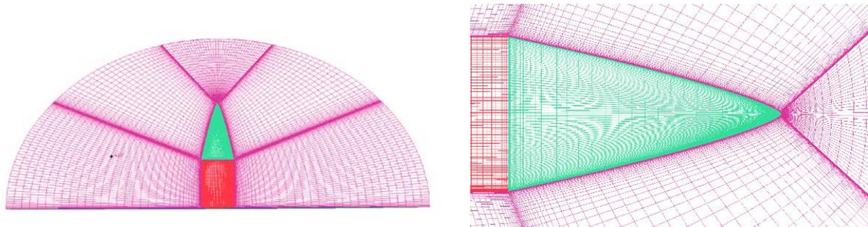
Figure 2 Structural mesh of outflow field
