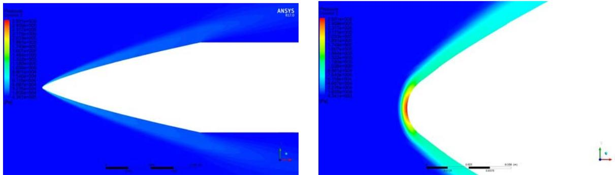
Figure 3 The distribution of flow field aerodynamic force
