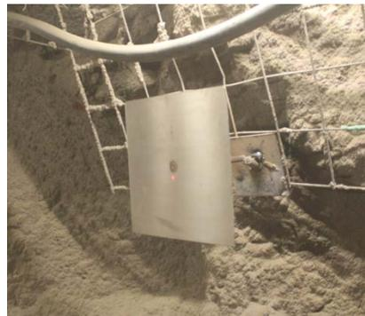
Fig. 8 Layout of the laser mark point
