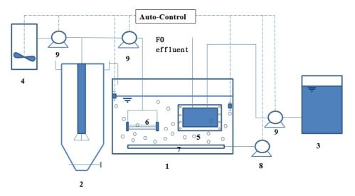
1 double membrane bioreactor ; 2 crystallization reactor ; 3 seawater draw solution ; 4 NaOH Dosing box ; 5 membrane module of forward osmosis ; 6 membrane module of ultrafiltration ; 7 aerator ; 8
