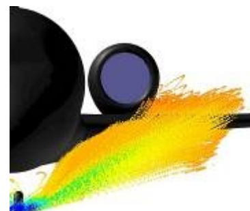
Fig. 5 Optimized chine tire spray trajectory in aircraft flowfield. (V=55m/s, H=16mm)
