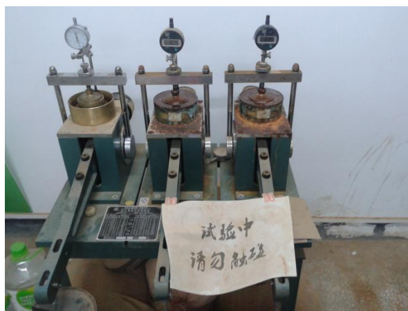
Fig. 1 WG high pressure consolidation apparatus
