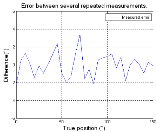
Fig. 12. Error between several repeated measurements
