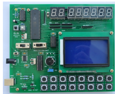
Fig. 1. The serial interface technology circuit board
