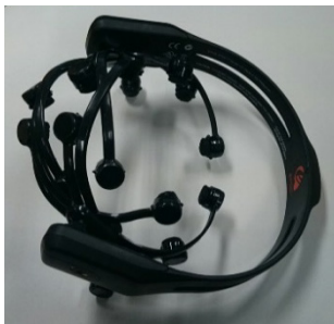
Fig. 1. Emotiv EPOC (wireless portable EEG headset)
