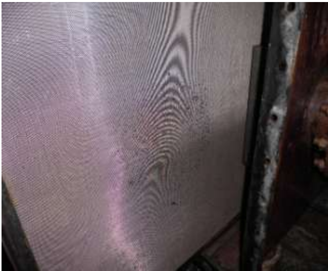
Fig. 11. Clogging of a mesh filter with large particulates
