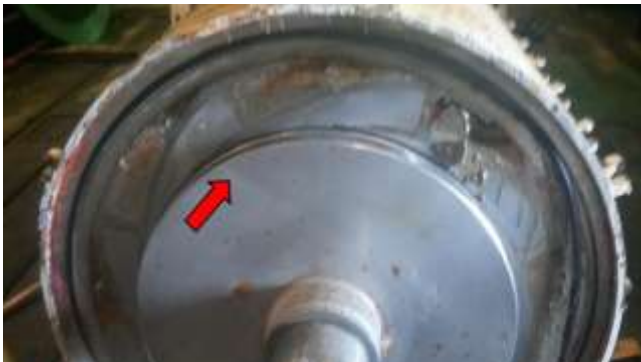
Fig. 4. Deformation of the impeller
