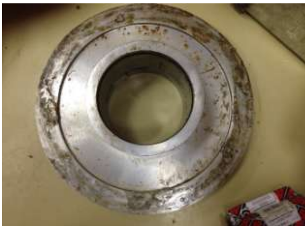
Fig. 5. Intensive hydroabrasive wear of the hydraulic balancing device disk
