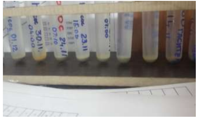
Fig. 6. Settled solid phase of mine waters at the Udachny mine under laboratorial conditions
