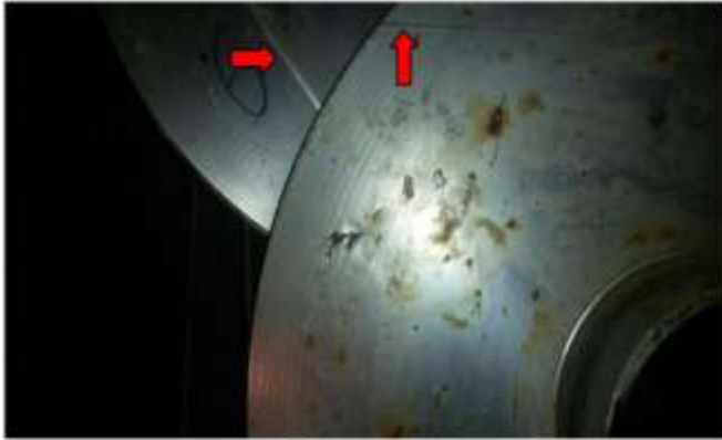
Fig. 3. Abrasive wear of the impellers
