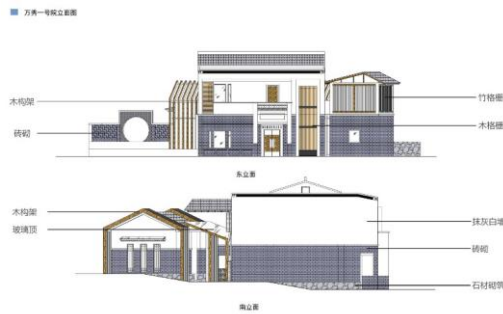
Fig. 8. Facade reconstruction of buildings in Wanxiu No. 1 courtyard.
