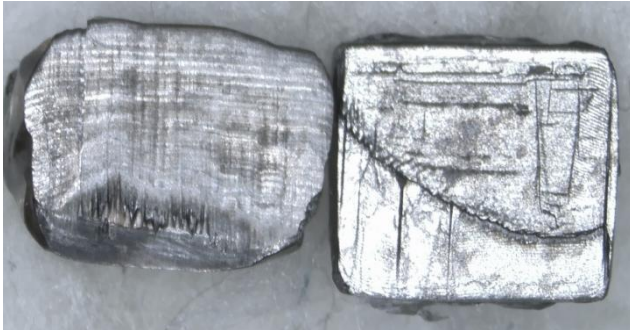
Figure 3. Laser cutting (left) and WJL cutting (right).
