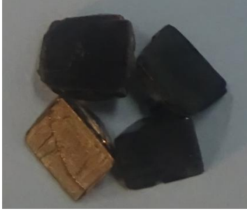
Figure 2. Samples cut by WJL and laser.
