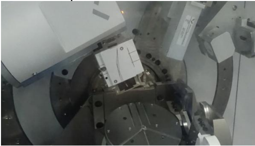
Figure 7. XRD test of the diamond cutting surface.
