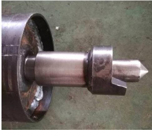
(a) male head butt joint structure
