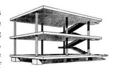
Shanghai Special Municipal Government Building was totally different, the original structure type could be traced back to Le Corbusier's Citroen residential structure system. There are three layers including floors lab, beam grid and column grid.
