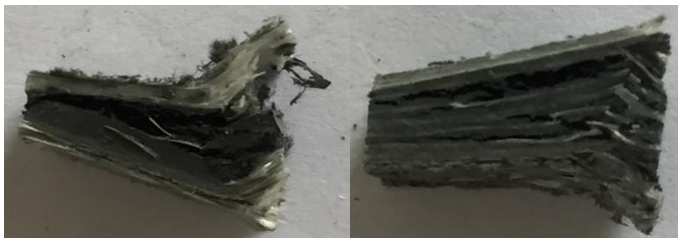
(a) B compressed fracture (b) C compressed fracture Fig.3 B、C compressed fracture
