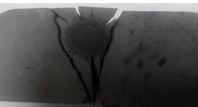
a-Al-3 wt% Y; b-Al-2.5 wt% Cu- 3 wt% Ti; c - destruction of the substrate Fig. 4. Graphite interaction with aluminum melts doped with carbide forming elements.
