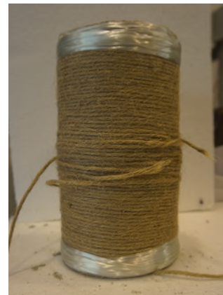
Fig. 6. Typical failure mode of R-2 specimen.
