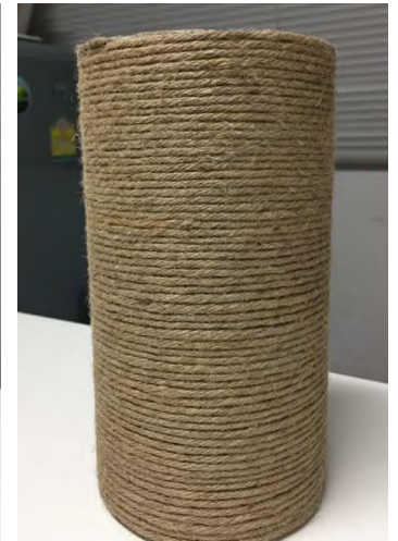
Fig. 3. A typical rope strengthened concrete specimen.
