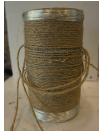
Fig. 5. Typical failure mode of R-1 specimen.
