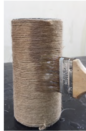
Fig. 3. Applying the epoxy resin using resin
