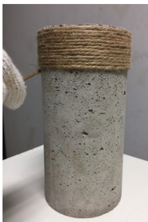
Fig. 2. Wrapping processes of dry rope to the concrete specimen.
