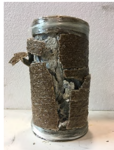
Fig. 7. Typical failure mode of RE-1 specimen.
