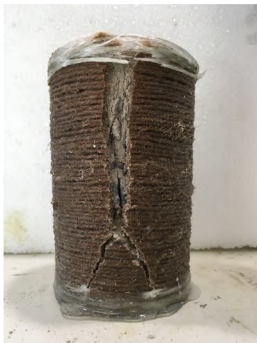
Fig. 9. Typical failure mode of RE-3 specimen.
